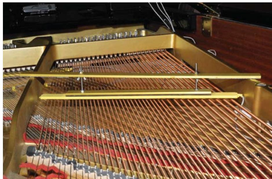
The pickup pedestals can be tweaked to reduce the almost painful amount of attack generated by hard-playing performers.
