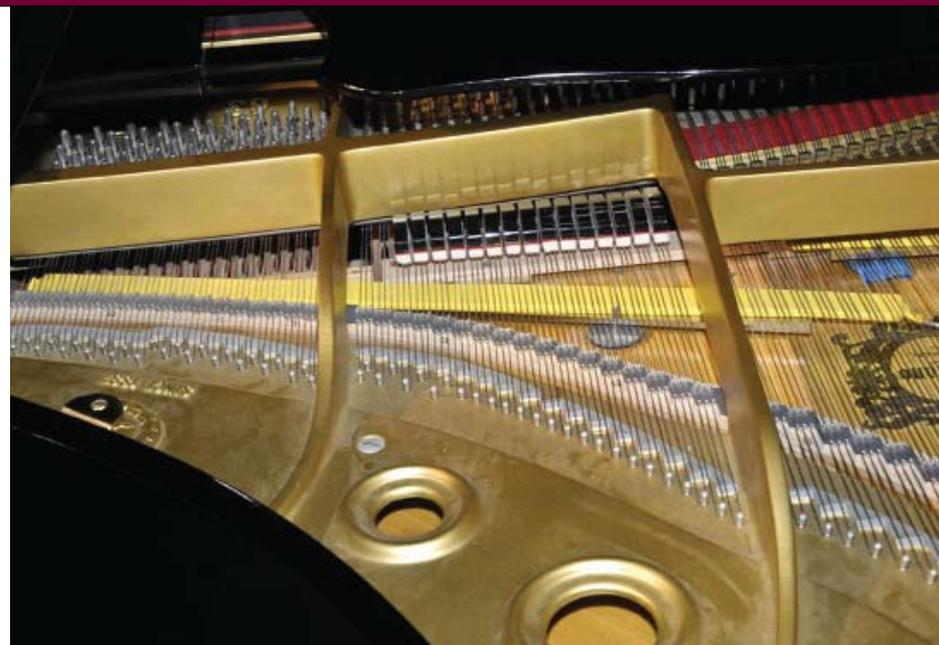
The Helpinstill Piano Sensor (yellow), includes three pickups, one for the high register, mid-register and low register.
