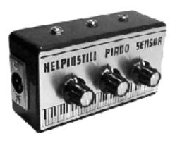
The control box is a passive unit. It does not require batteries, phantom power, or any other power source. This means it is compatible with sound systems worldwide, and requires no maintenance. The XLR connector provides an output at mic level, while the 1/4" jack high-impedance output is comparable to that of an electric guitar.
