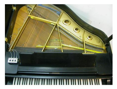
The silver support bars are used to support two sensors under the middle and treble strings. The gold double support bar suspends the third sensor over the bass strings.
