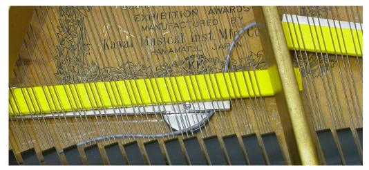
When removing these units from the piano it is perfectly okay to use the wires to pull them out of the piano. These wires are very strongly attached inside the sensors and nearly impossible to pull loose.
