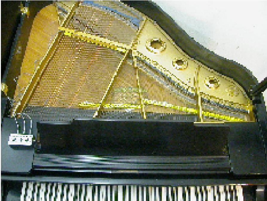
The silver support bars are used to support two sensors under the middle and treble strings. The gold double support bar suspends the third sensor over the bass strings. Before installing any of the pickup strips, remove the tie wraps from the gray cables and **smooth out, stretch and straighten the cables**. If they kink and curl under the strings, they may touch them and cause a buzzing noise.
